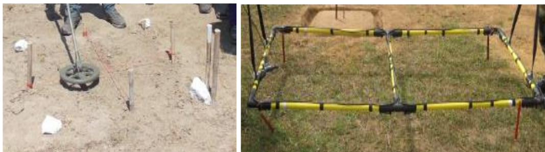
Figures 20 and 21: Example - Performance test of metal detector and UXO detector (Photos provided by Doug Ware, UNMAS)
