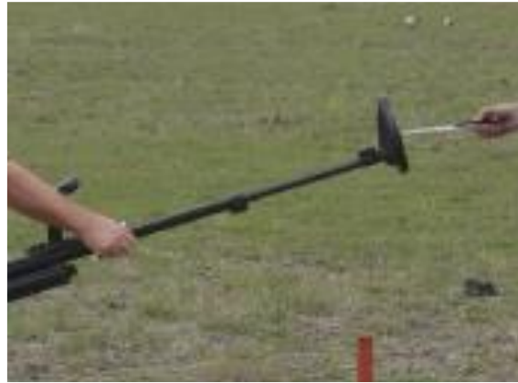
Figure 23: Example - Detector confirmation test using manufacturer's test piece and ruler (Photo of provided by Doug Ware, UNMAS)
